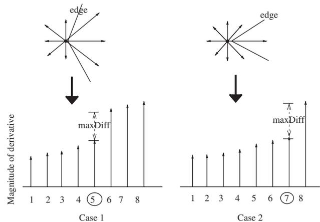
Fig. 3. Discarding redundant interest points. The indices of maximum difference in the two cases are 5 and 7, respectively.
