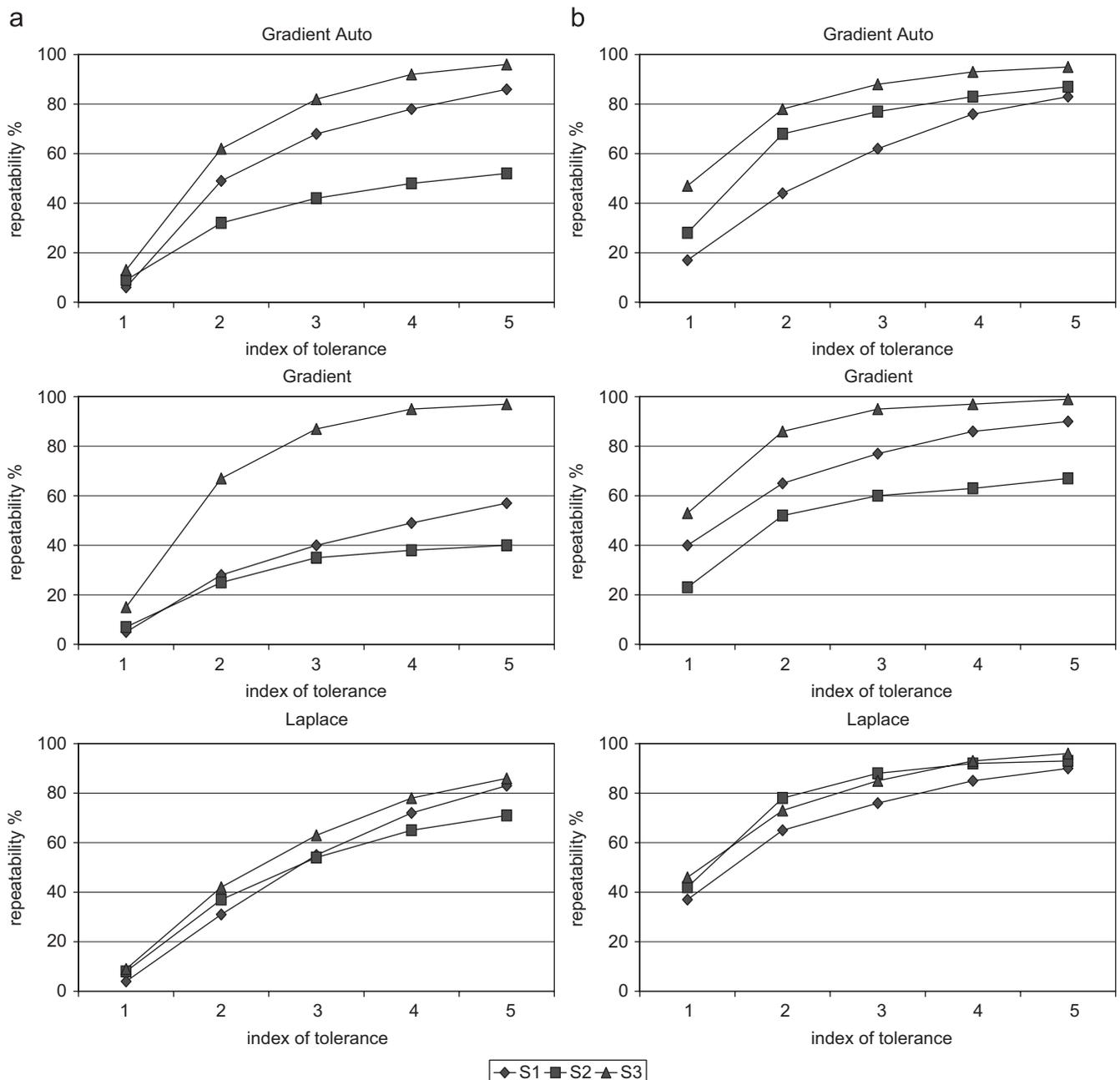
Fig. 9.  $\epsilon$ -repeatability rates of nine detectors with respect to localization tolerances (from  $\epsilon_1 = 0.5$  to  $\epsilon_5 = 4.5$ ): (a)  $\theta_1 = -45^\circ$  and (b)  $\theta_5 = -5^\circ$ .
