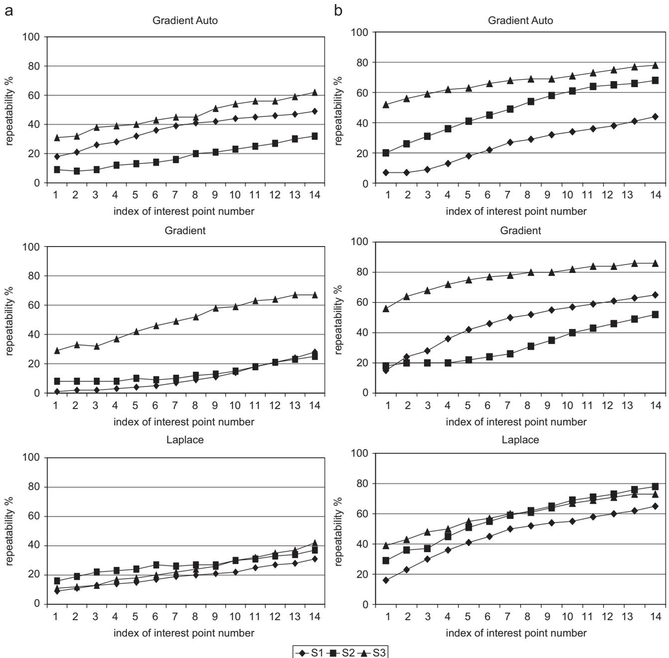
Fig. 10.  $\varepsilon_2 = 1.5$ -repeatability rates of nine detectors with respect to interest point numbers (from  $n_1 = 140$  to  $n_{14} = 400$ ): (a)  $\theta_1 = -45^\circ$  and (b)  $\theta_5 = -5^\circ$ .
