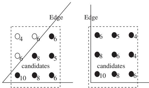
Fig. 1. Non-maximum suppression destroys the geometric structure.
